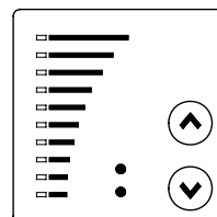
Fig. 20 Control panel of a CME pump
